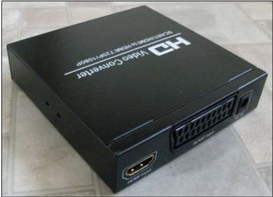
SCART to HDMI video converter unit
