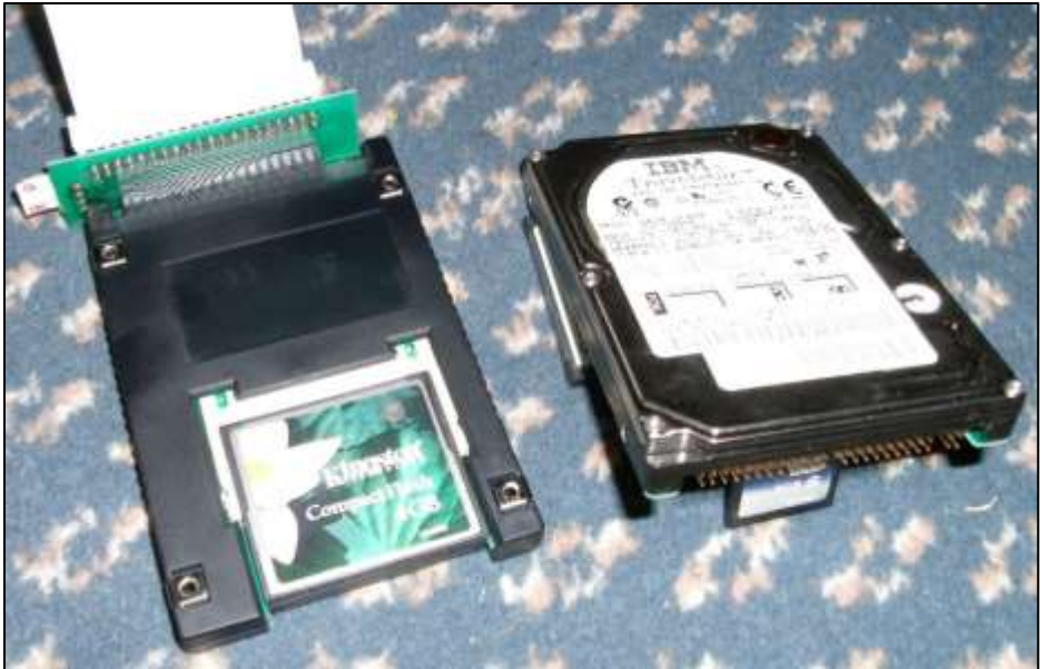
The Syba 2.5 inch dual CF card adaptor, shown alongside a typical 2.5 inch hard drive. The Syba unit is shown with the small 40 to 44 pin connector adaptor PCB at the rear.
