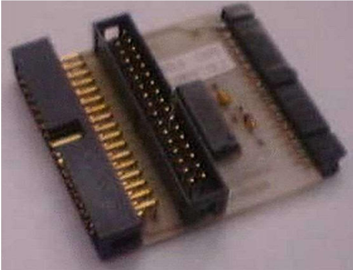
*Figure 1 – The 4-drive adapter for Gold Card, from Miracle Systems*
